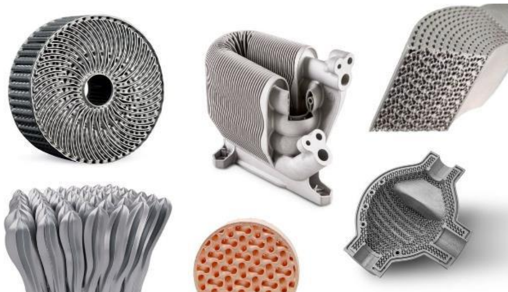
Figure 23: Complex near-net shape metal 3D printed heat exchangers with internal structures unachievable via traditional manufacturing methods. Since the surface area to volume ratio and position of that surface area relative to air flow are critical in heat exchanger efficiency, 3D printing allows step change increases in performance over traditional heat exchangers (source: https://all3dp.com/1/better-heat-exchangers-with-additive-manufacturing/ ).
