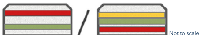
Figure 15: Multiple layered particles with different physical characteristics in each layer (source: Gooch, Daniel, et al. , 2016).
